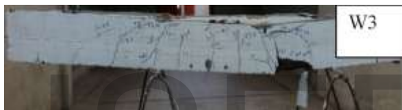
Fig. 11–Pattern of cracks of beam (W3).
