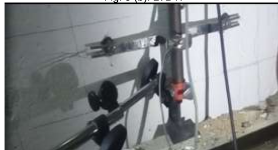
Fig. 5 (C). Crack width measurement device.
